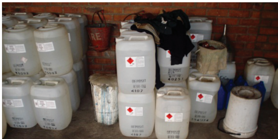
Illegal storage of flammable liquids
